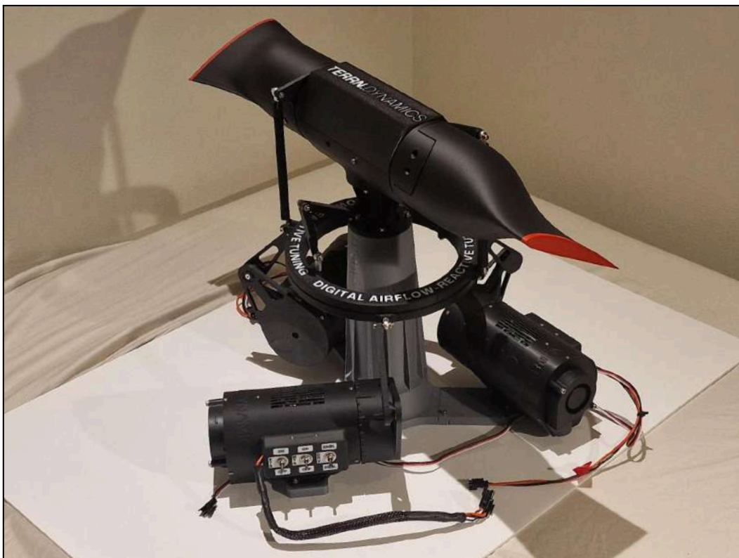
Fig. 5.1B, Photo of the DART Prototype, Note Inaccurate Propeller Blade Orientation
